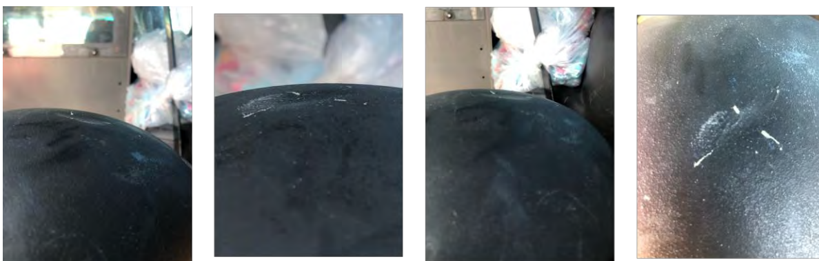
Figure 59. Damage to Officers' Helmets
