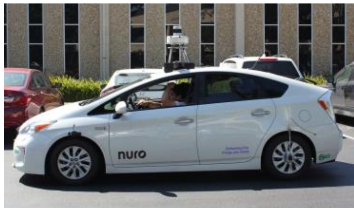
The Nuro Autonomous Prius looks similar to a traditional consumer Toyota Prius with additional hardware mounted on the top of the vehicle. It is monitored by an In-Vehicle Safety Operator and can be manually driven if necessary. The vehicle has a [REDACTED] and will only operate on roadways with a posted [REDACTED]. Proof of insurance and registration can be provided by the In-Vehicle Safety Operator. After conducting a vehicle stop on the Nuro Autonomous Prius vehicle, the In-Vehicle Safety Operator will disable the autonomous mode and the officer can safely approach the vehicle for interaction with the In-Vehicle Safety Operator.
